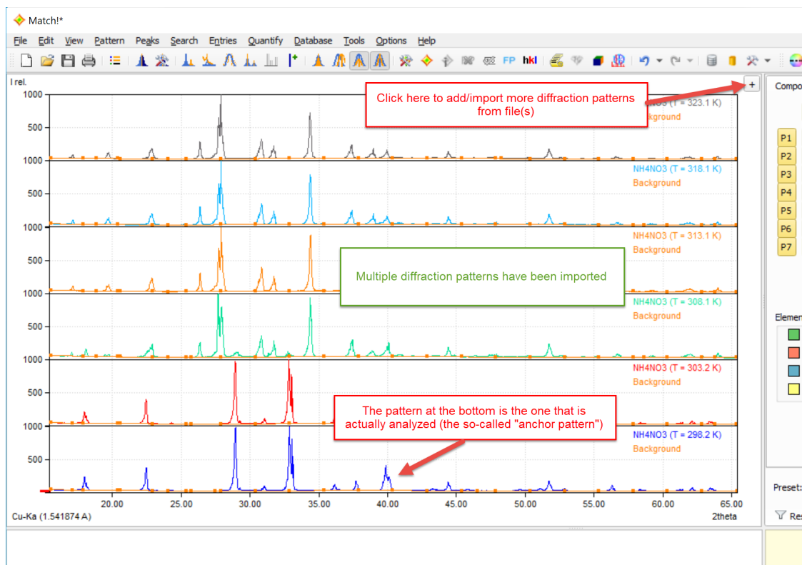
Fig. 71: Six experimental diffraction patterns are stacked on top of each other.
